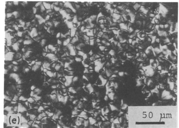
Figure 3 Polarized light micrographs of carbons obtained from mixtures of fractionated pitches and PVC under pressure. (a) PF-1, (b) PF-1 + 10% PVC, (c) PF-1 + 30% PVC, (d) PF-1 + 90% PVC, (e) PF-3 + 10% PVC.
